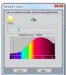
Step 5. To make a dark measurement cover the sensor or turn off the calibration source so the dark reference spectra can be measured. Click next and the calibration is finished.
