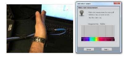
When you close the calibration dialog will you be asked if you want to save the calibration to the device. When selecting yes the custom calibration will be saved inside the device. You can switch back to the factory calibration at any time.
