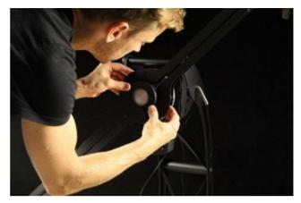
Then place the sensor approximately two meters away (recommended to use approximate same distance as defined on certificate) from the setup with the reference lamp. Make sure the sensor is aligned with the lamp. Shoot the laser towards the lamp glass and catch the reflected beam in the same area of its origin, or within a 4 cm area. Such a procedure puts both the sensor and the lamp in alignment. The pictures below explain the process:
