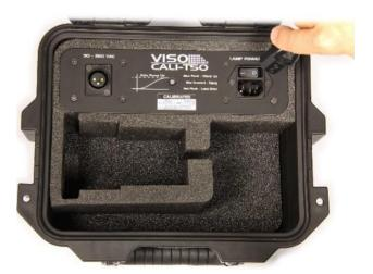
The lamp needs to ramp up, and there is an indicator with a mini instruction on the box. The blue flashing indicator means the lamp is ramping up, a constant blue colour defines the lamp is ramped up, whereas the red colour of the indicator means there is an error.
