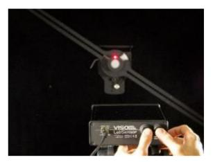
The glass surface of the lamp produces a lot of internal reflections of the laser beam, and it complicates the exact distance calculation. The precise distance determination is essential in achieving the best results. That is why a fixed white target point was designed above the lamp luminous area.
